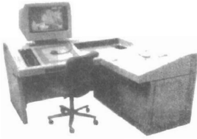
Figure 2-39 An artist's workstation, featuring a color raster monitor, keyboard, graphics tablet with hand cursor, and a light table, in addition to data storage and telecommunications devices. (Courtesy of DICOMED Corporation.)
