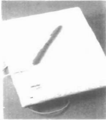
Figure 2-48 The NotePad desktop tablet with stylus. (Courtesy of CalComp Digitizer Division, a part of CalComp, Inc.)
