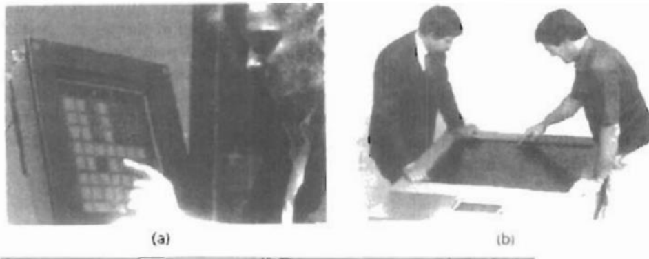
Figure 2-54 Plasma panels with touch screens. (Courtesy of Photonics Systems.)
